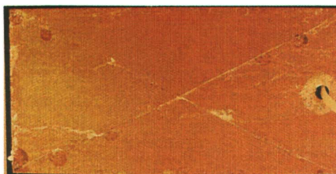
Plate 9. Scribed polymer coated Al panel (1146 hours of exposure). (Reproduced from reference 12.)
