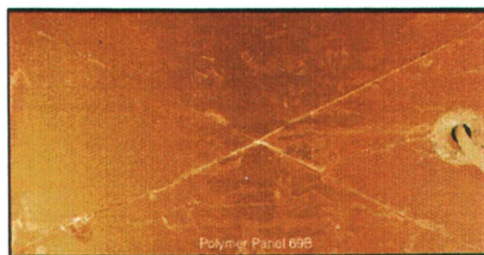
Plate 7. Scribed polymer coated Al panel after 616 hours of exposure. (Reproduced from reference 12.)
