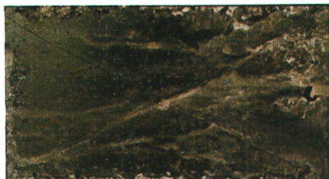
Plate 12. Scribed conversion coated Al panel (3000 hours of exposure). (Reproduced from reference 12.)
