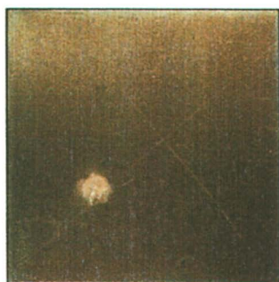
Plate 3. Panel 3. 3% BAMPPV/epoxy coating on aluminum substrate.
