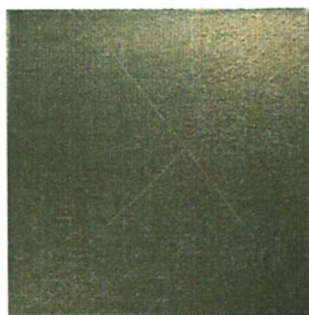
Plate 2. Panel 2. Pure epoxy coating on aluminum substrate.
