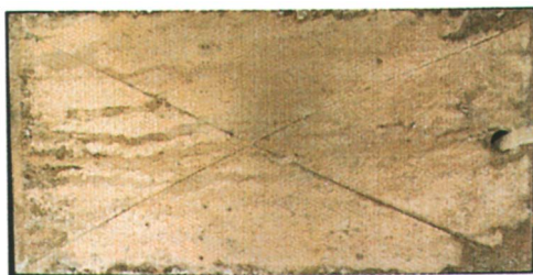
Plate 10. Scribed conversion coated Al panel (1146 hours of exposure). (Reproduced from reference 12.)
