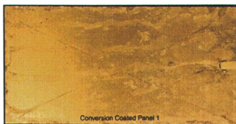
Plate 8. Scribed conversion coated Al panel after 616 hours of exposure. (Reproduced from reference 12.)
